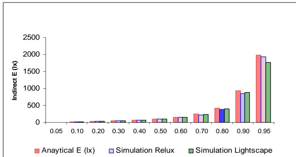
Figure 20: Simulation results for the diffuse inter-reflections test case
