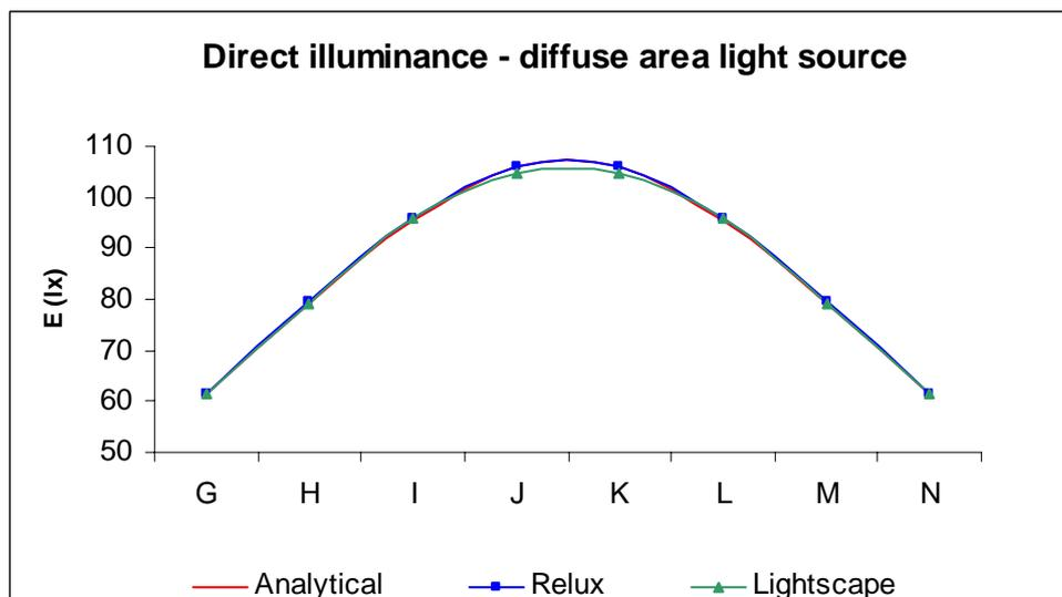
Figure 4: Simulation results at floor reference points for area light source scenario with diffuse photometry
