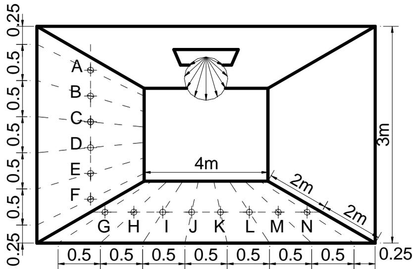
Figure 3: Scenario description for area light source test case
