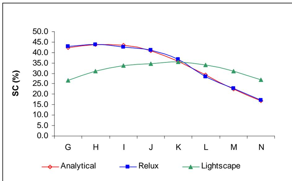
Figure 12: Simulation results at floor reference points in SC for 4m×4m roof unglazed opening and a CIE clear sky (General sky Type 12)
