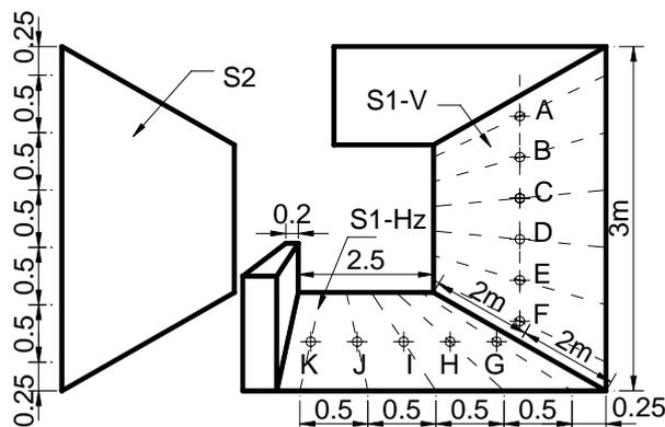
Figure 18: Scenario description for diffuse reflection with obstruction
