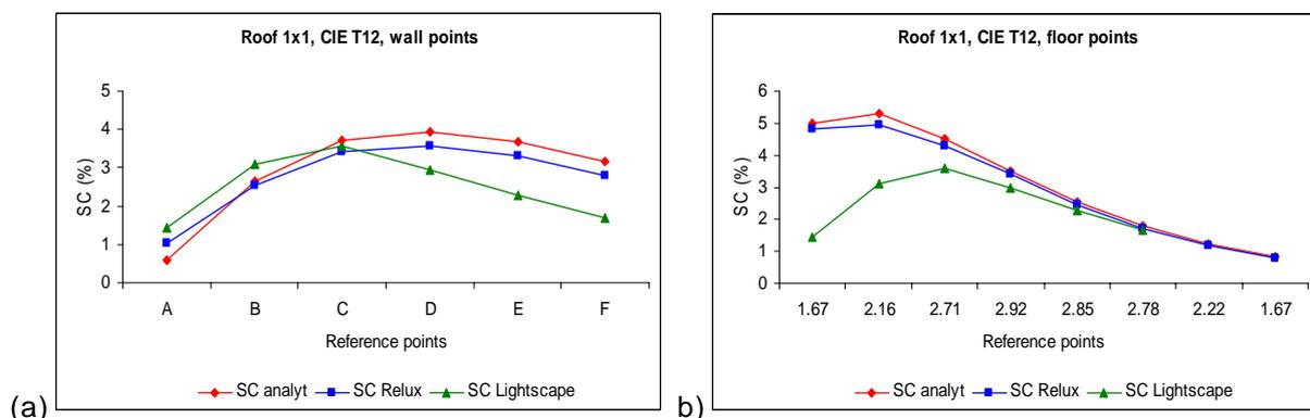
Figure 13: Simulation results in SC for 1m×1m roof glazed opening and a CIE clear sky (General sky Type 12). (a) shows results at wall reference points and (b) shows results at floor reference points.
